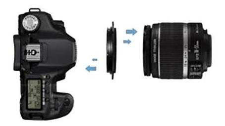
The one drawback with using a reversing ring with a Canon camera is that there is no manual method of closing down the aperture. There are two ways around this. The first method, one not recommended by Canon, is to firstly set the camera on AV mode, set the desired aperture with the lens the right way round and then press the depth-of-field preview button. Next, with the
